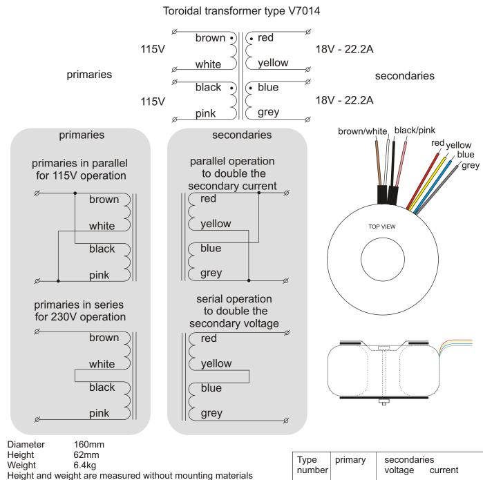
Height and weight are measured without mounting materials All leads are solid and approx 200mm long
