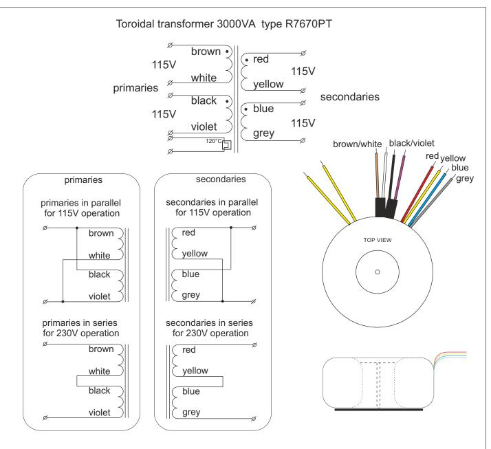
Built-in selfresetting thermal cut-out 120°C to be applied in auxiliary circuits only!
