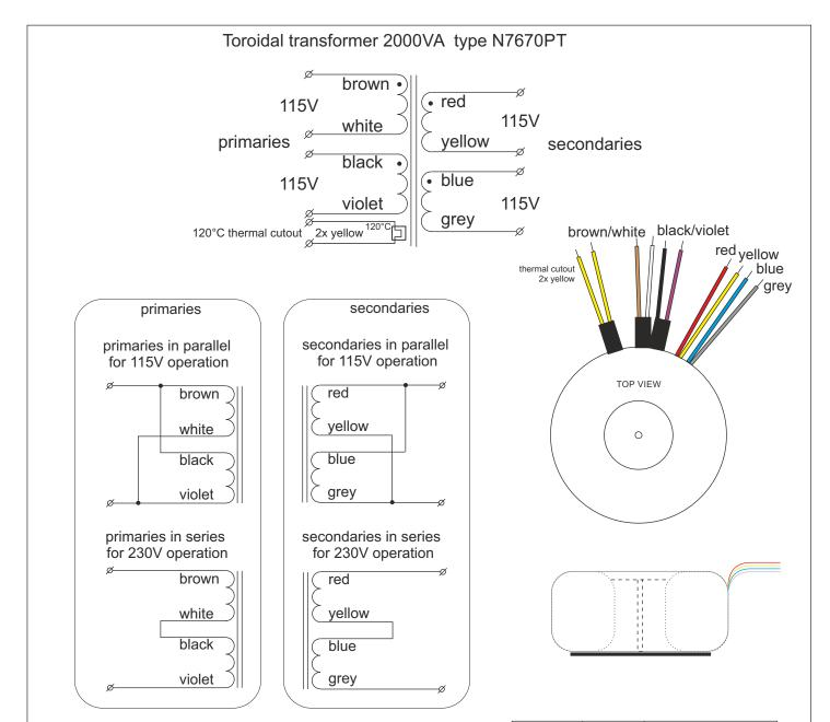
Built-in selfresetting thermal cutout : 120°C to be applied in auxiliary circuits only !
