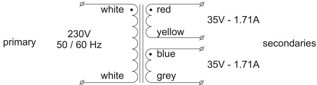
serial operation to double the secondary voltage
