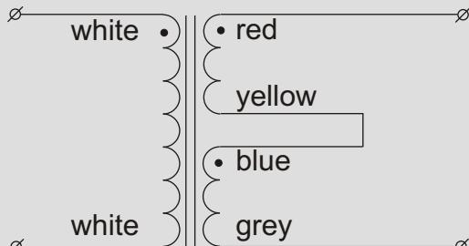
parallel operation to double the secondary current
