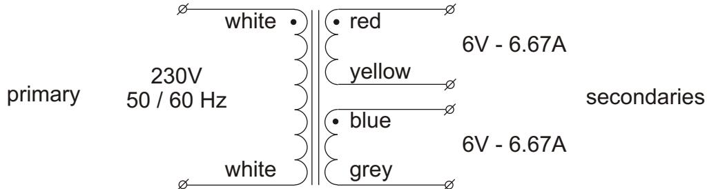
serial operation to double the secondary voltage
