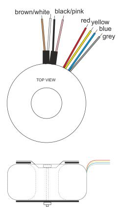
Diameter 70mm Height 32mm Weight 0.44kg
