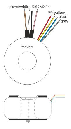
Diameter 70mm Height 32mm Weight 0.44kg
