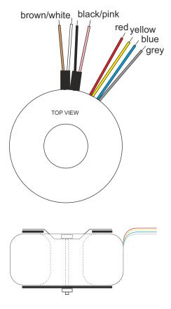
Diameter 70mm Height 32mm Weight 0.44kg
