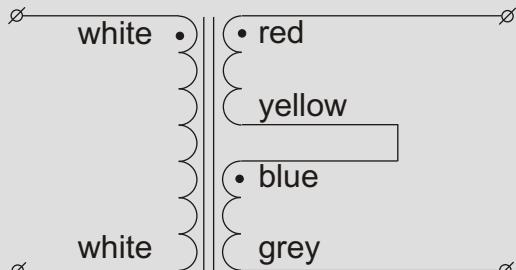
parallel operation to double the secondary current
