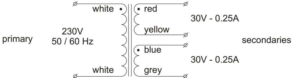
serial operation to double the secondary voltage
