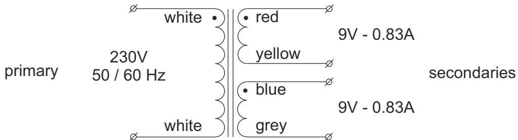
serial operation to double the secondary voltage
