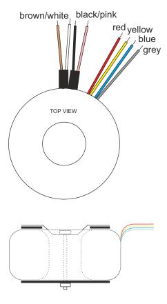
Diameter 60mm Height 28mm Weight 0.31kg
