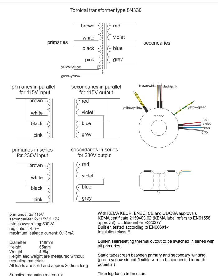
Supplied mounting materials: 1 metal washer Ø11cm 2 neoprene washers Ø11cm 1 bolt M8x70 with nut
