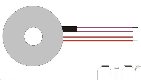
Toroidal transformer: Power rating: 625VA
