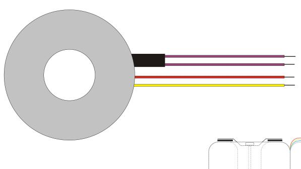
Toroidal transformer: Power rating: 120VA
