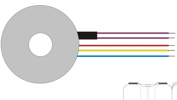
Toroidal transformer: Power rating: 48VA
