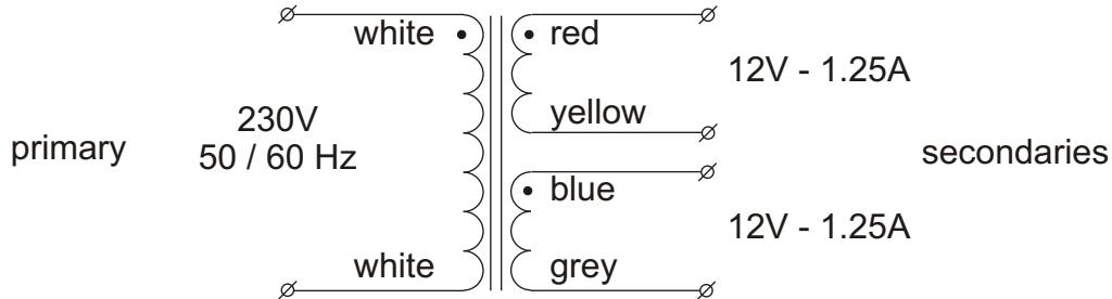
serial operation to double the secondary voltage
