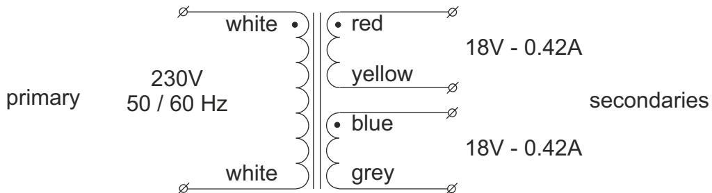
serial operation to double the secondary voltage
