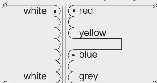
parallel operation to double the secondary current
