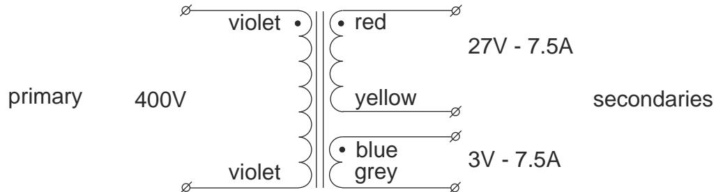
serial operation to increase the secondary voltage
