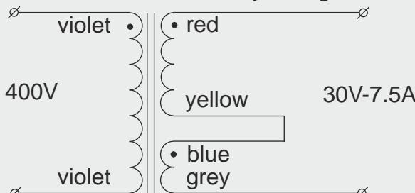
parallel operation to double the secondary current
